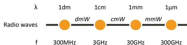
As indicated above, the propagation properties at these frequencies will have to be carefully characterized in order to select appropriate spectrum and system design. For instance, the penetration loss of a mmW signal as well as the higher free-space path loss (i.e. line of sight atmospheric path) at these frequencies due to smaller antennas, both require the use of antenna(s)
