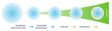
Figure 6. Cellular topology evolution towards more capacity (and better coverage)
